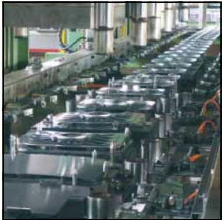
◀ Transferlinie Progressive die with grabber transfer
